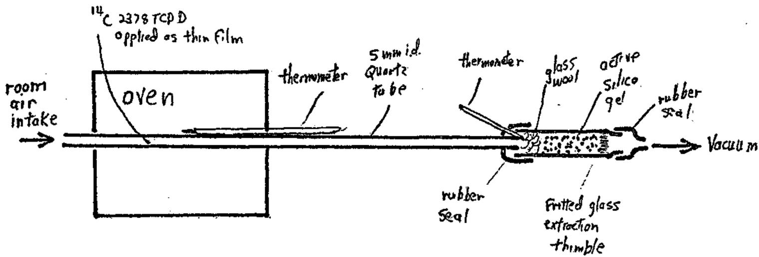
Figure 1. TCDD Volatilization and Trapping Apparatus
