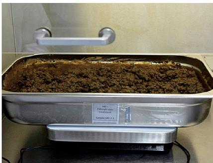
Fig.1: Treated Soil Layers of 10 – 15 cm (Photo by HPC, 2014)
