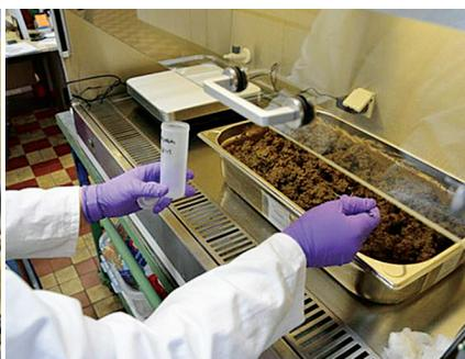
Fig.4 a, b & c: Measuring of pH and Redox (Eh) (Photo by HPC, 2014)
