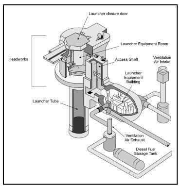
Figure 3.1-1. Launch Facility Schematic
