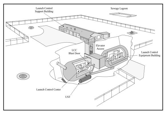
Figure 3.1-3. Missile Alert Facility Schematic
