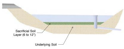
Figure 15. Schematic illustration of a sacrificial soil layer.
