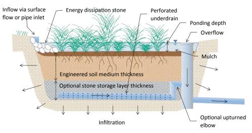
Figure 11. Example schematic design profile appropriate for use in feasibility analysis.
