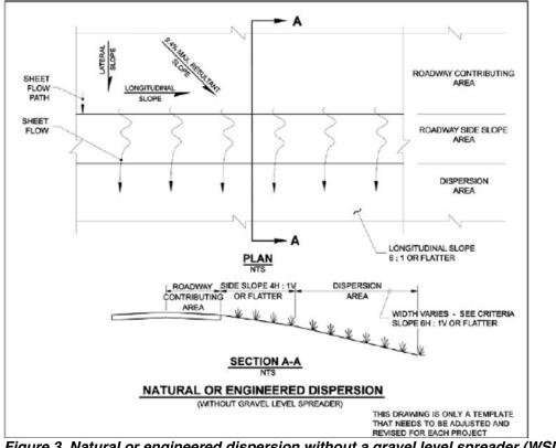
Figure 3. Natural or engineered dispersion without a gravel level spreader (WSDOT 2014).
