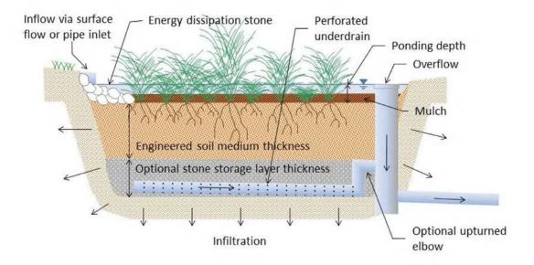
Figure 1. Cross-section view—upturned elbow.
