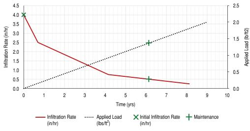
*Figure 14. Example results from roadside BMP Clogging Risk Assessment Tool for infiltration rate reduction and applied load over time.*
