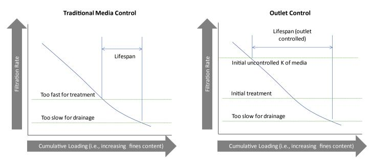
Figure 17. Schematic illustration of the lifespan benefits of outlet control.
