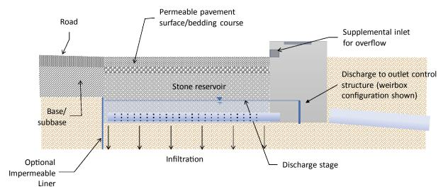
Figure 1. Cross-section view—urban setting with weir box.
