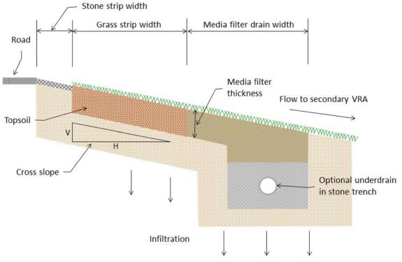
Figure 1. Cross-section view.
