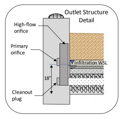
WSL: water surface level. *Figure 2. Example design of outlet control structure.*
