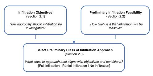
*Figure 5. Overview of methodology for preliminary selection of infiltration class.*
