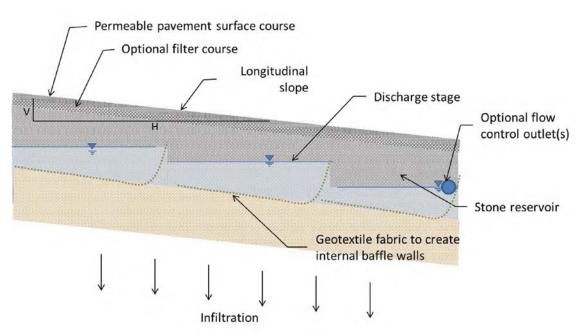
Figure 5. Longitudinal profile of an installation along a mild slope (geotextile cutoff walls).
