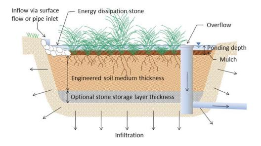
Figure 1. Cross-section view.
