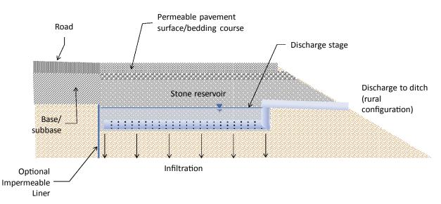
Figure 2. Cross-section view—rural setting with upturned elbow.
