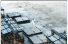
this contract, Parsons treated the excavated 15,000 tons of soil contaminated with Agent Orange and 15,000 tons of soil contaminated with PCBs and/or heavy oils. The thermal treatment included screening of all soil and briquetting the fine-particle soil prior to treatment. This contract also required that Parsons put into operation an extensive air emission treatment system along with a wastewater treatment plant that was also required under the thermal treatment contract.
