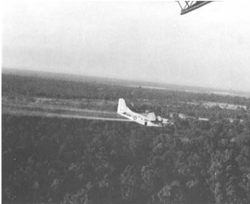
Top: an insecticide spray boom on the wing of a C-123; bottom: a Ranch Hand aircraft on an insecticide mission.
