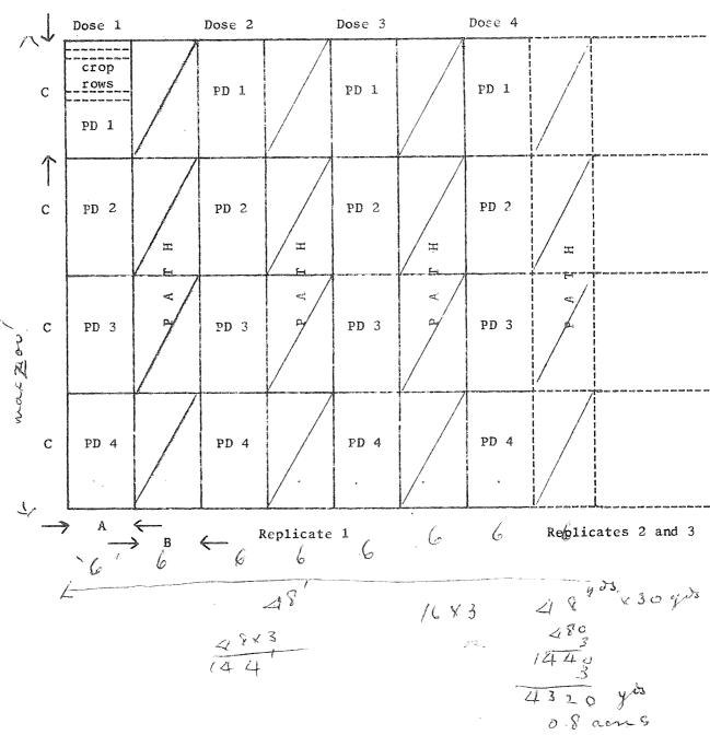
A - plot width determined by swathe width of sprayer butnot less than 6 ft
