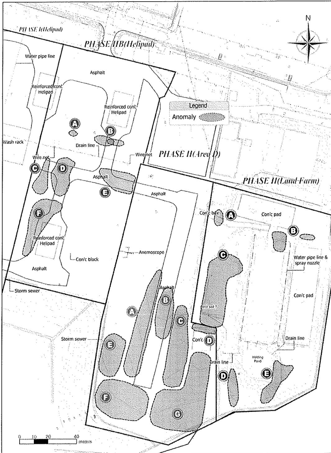
Figure 4-10 Combined Geophysical Survey Results Showing Subsurface Anomaly at Phase II/IIB Area.
