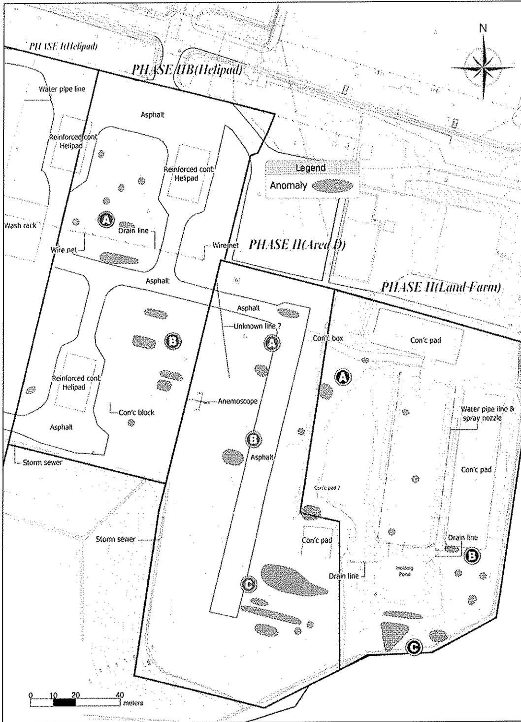
Figure 4-9 ERI Survey Result at Phase II/IIB Area.
