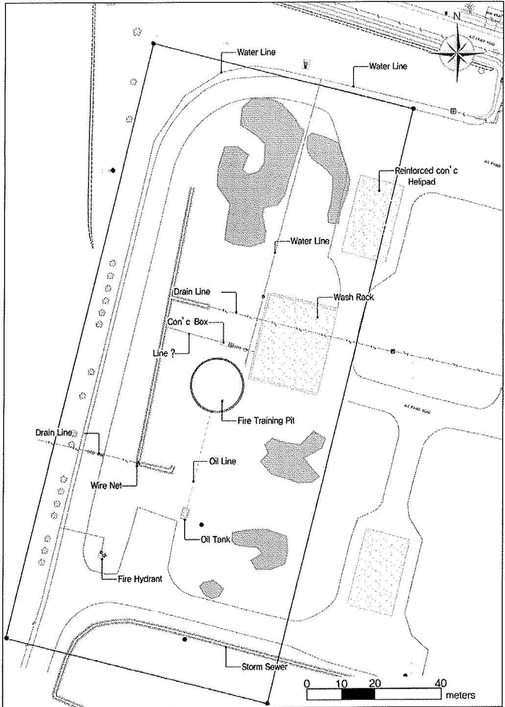
Figure 4-4 GPR Survey Result at Phase I of Helipad Area.
