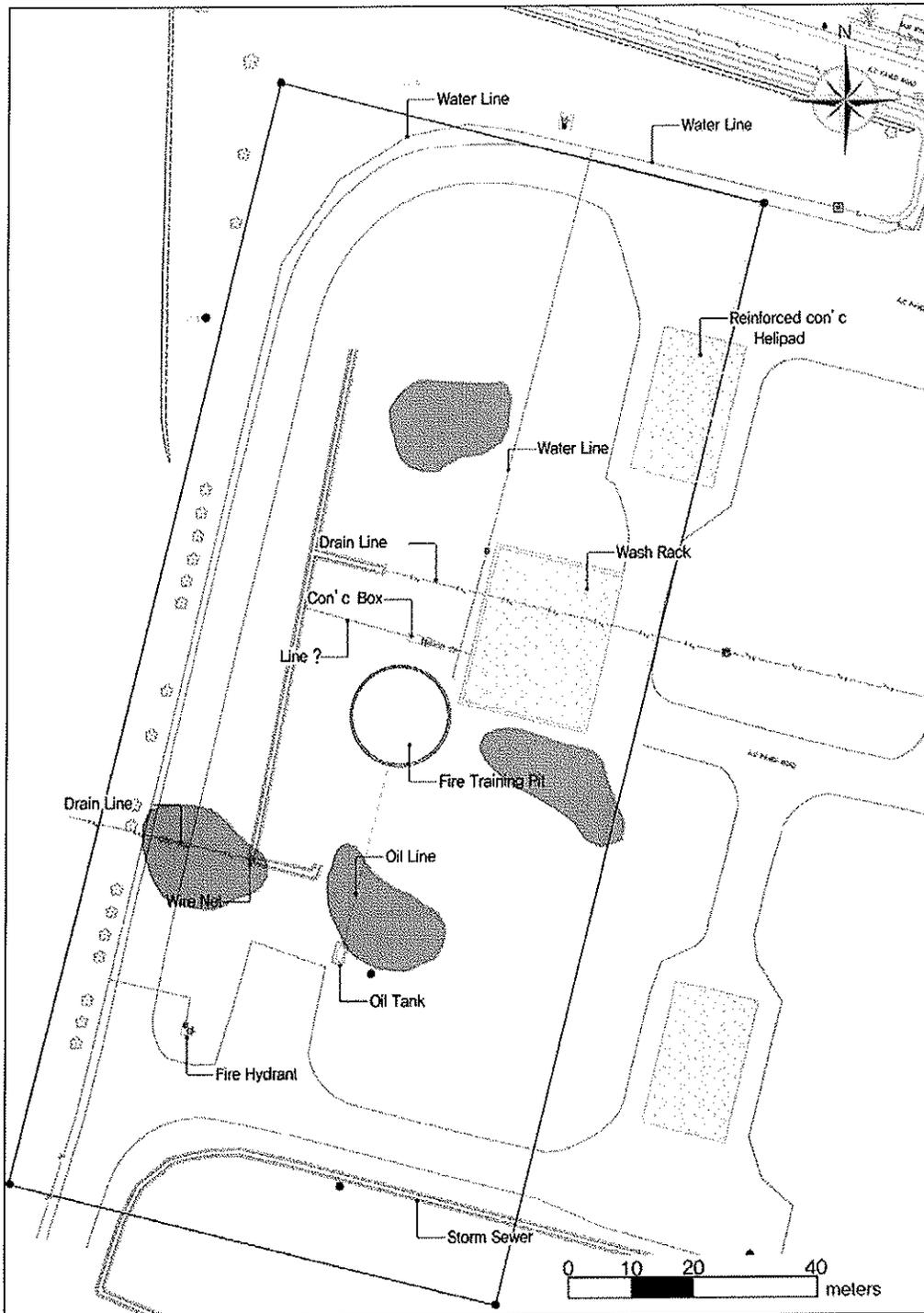
Figure 4-6 Combined Geophysical Survey Results Showing Subsurface Anomaly at Phase I of Helipad Area.
