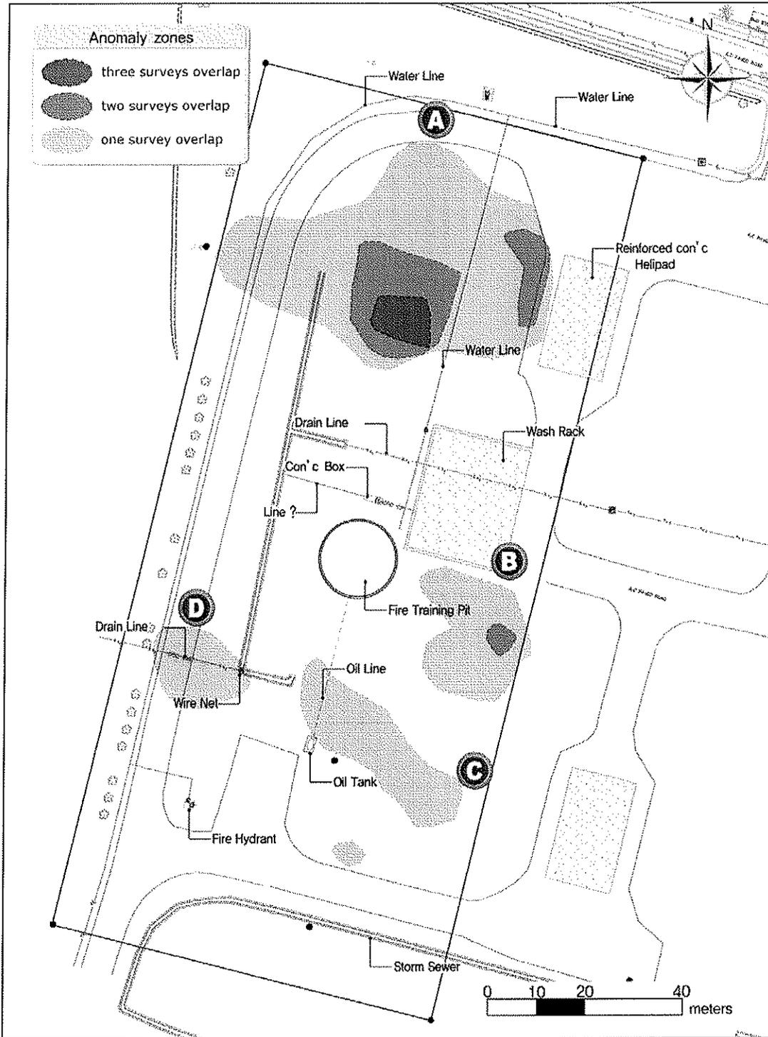
Figure 4-7 Magnetic Gradiometry Survey Result at Phase II/IIB Area.
