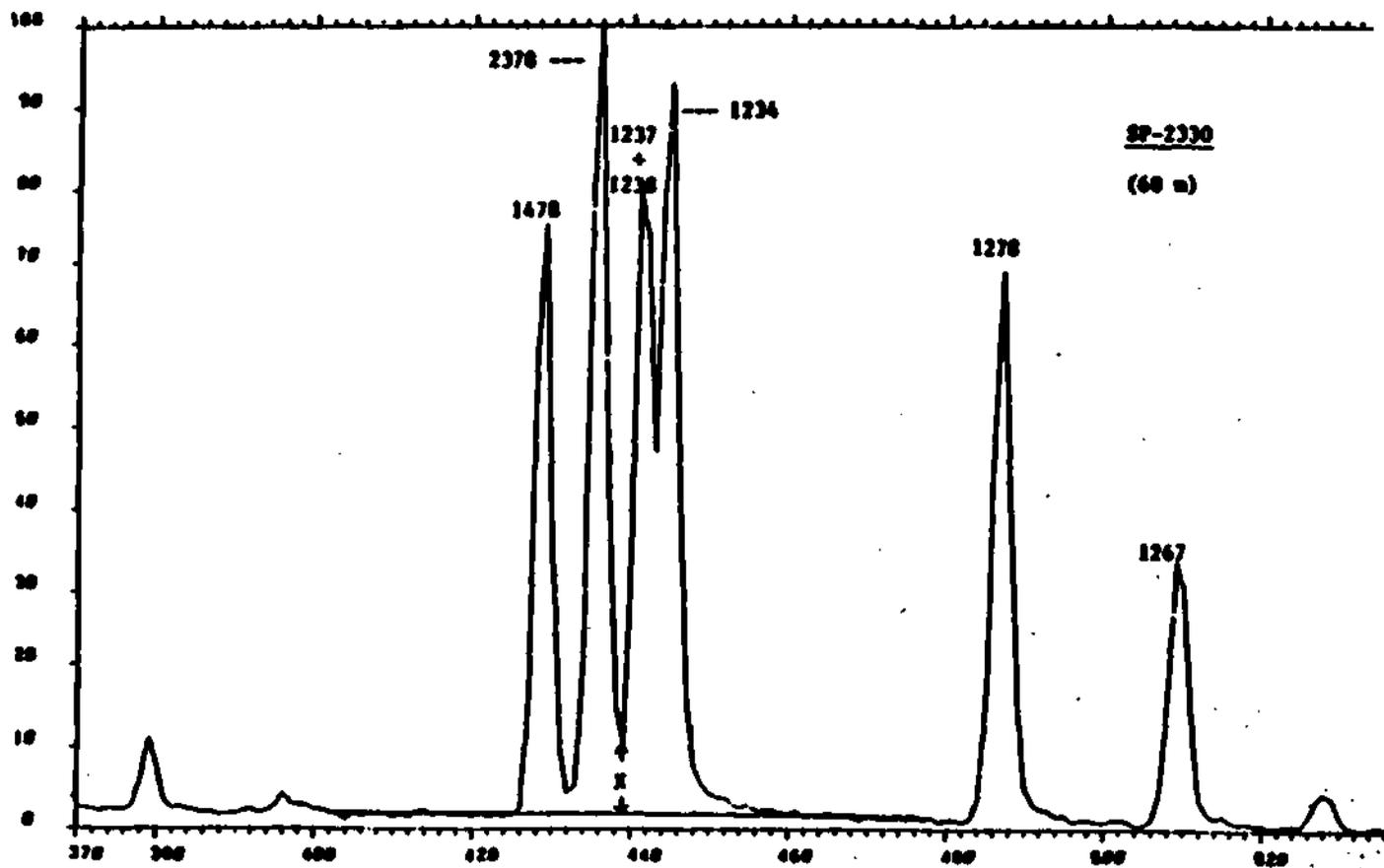
Figure 2. Selected ion current profile for  $m/z$  320 and 322 produced by MS analysis of performance check solution using a 60-m SP-2330 fused silica capillary column and conditions listed in Table 2.
