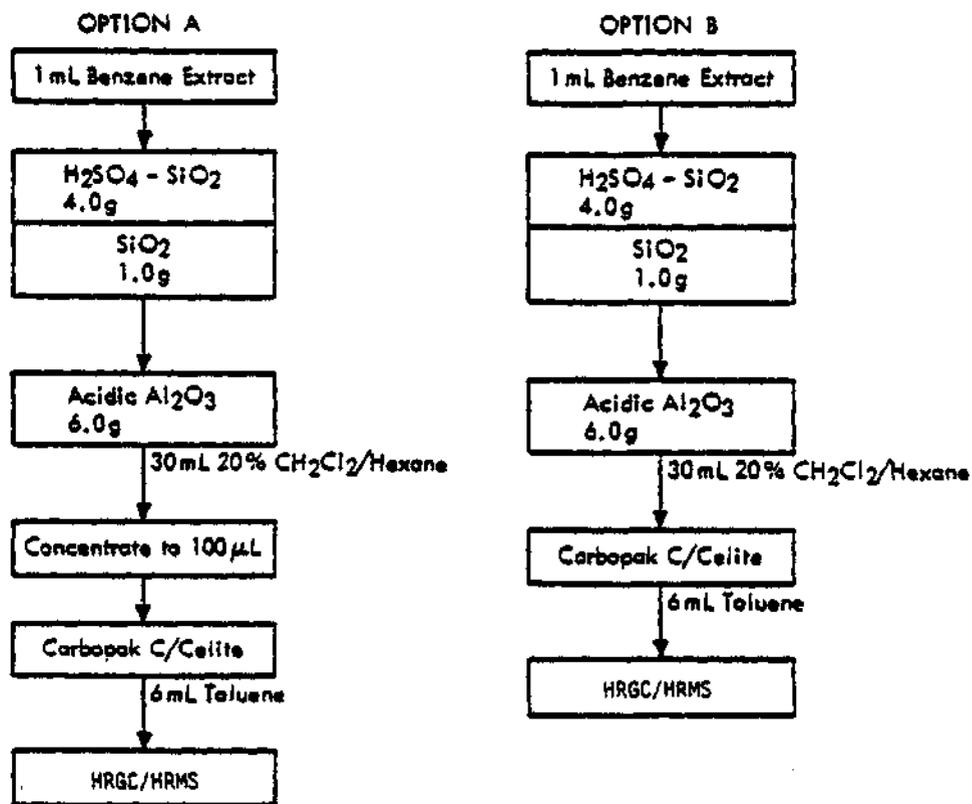
Figure 1. Column cleanup procedures specified in the protocol.
