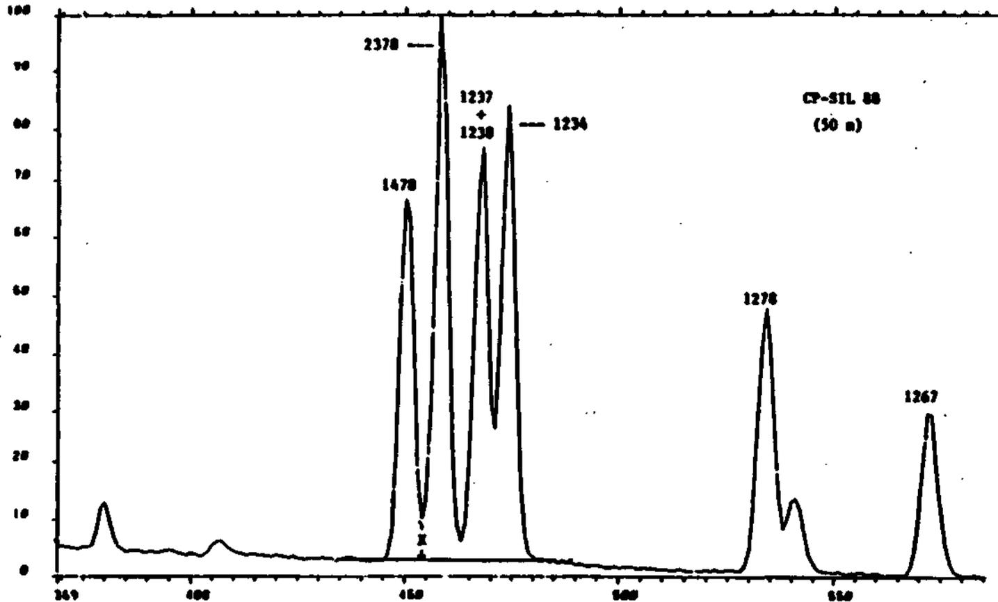
Figure 1. Selected ion current profile for  $m/z$  320 and 322 produced by MS analysis for performance check solution using a 50- $\mu$  CP Sil-88 fused silica capillary column and conditions listed in Table 2.
