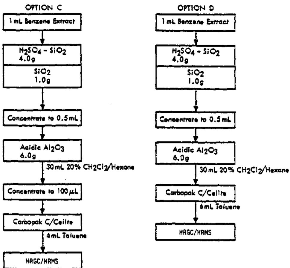
Figure 2. Column cleanup procedures proposed by the EMSL-LV.
