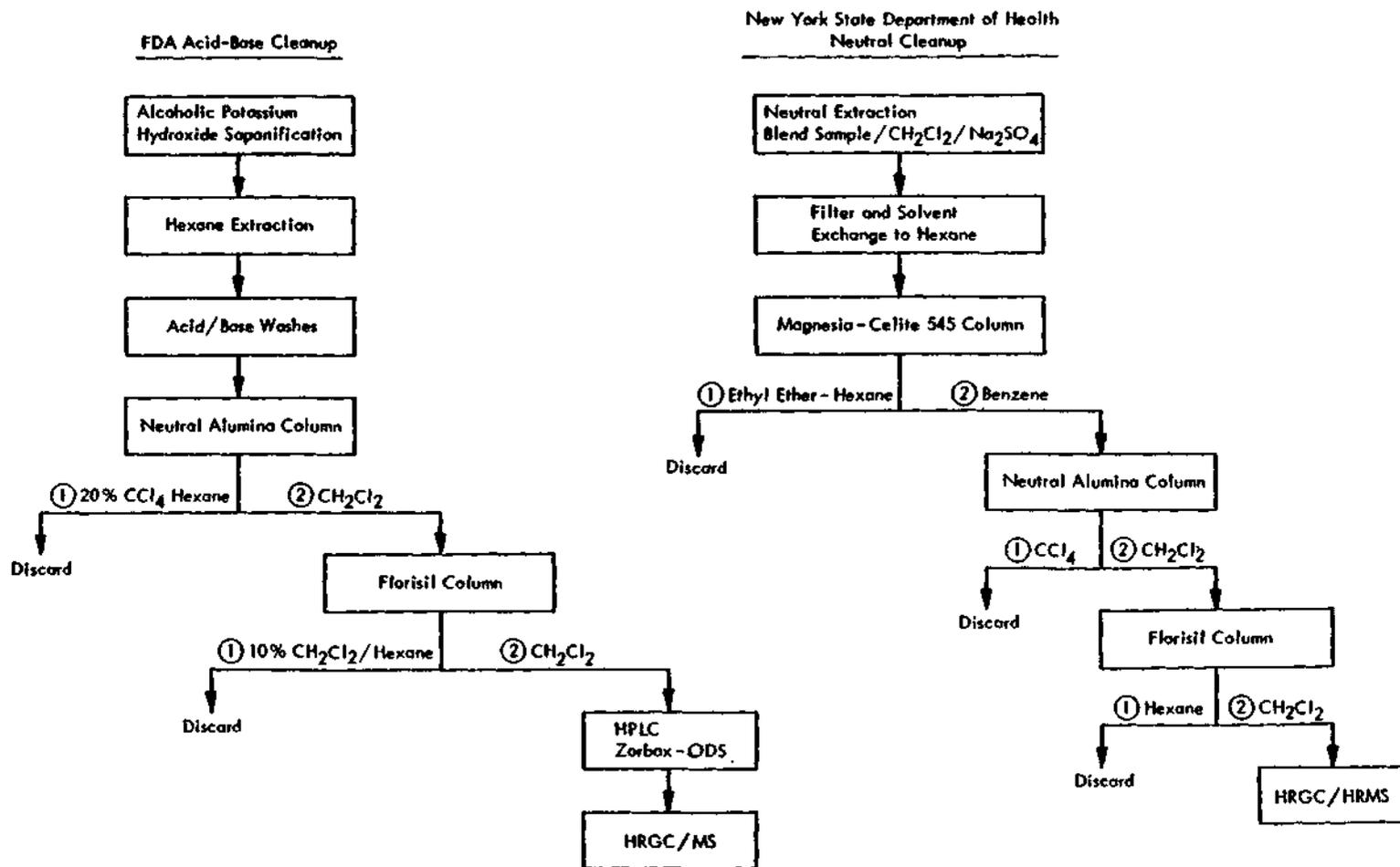
Figure 3. Schematic presentation of the sample preparation schemes used by FDA and laboratories and the New York State Department of Health in collaborative study of fish sample preparation and analysis.
