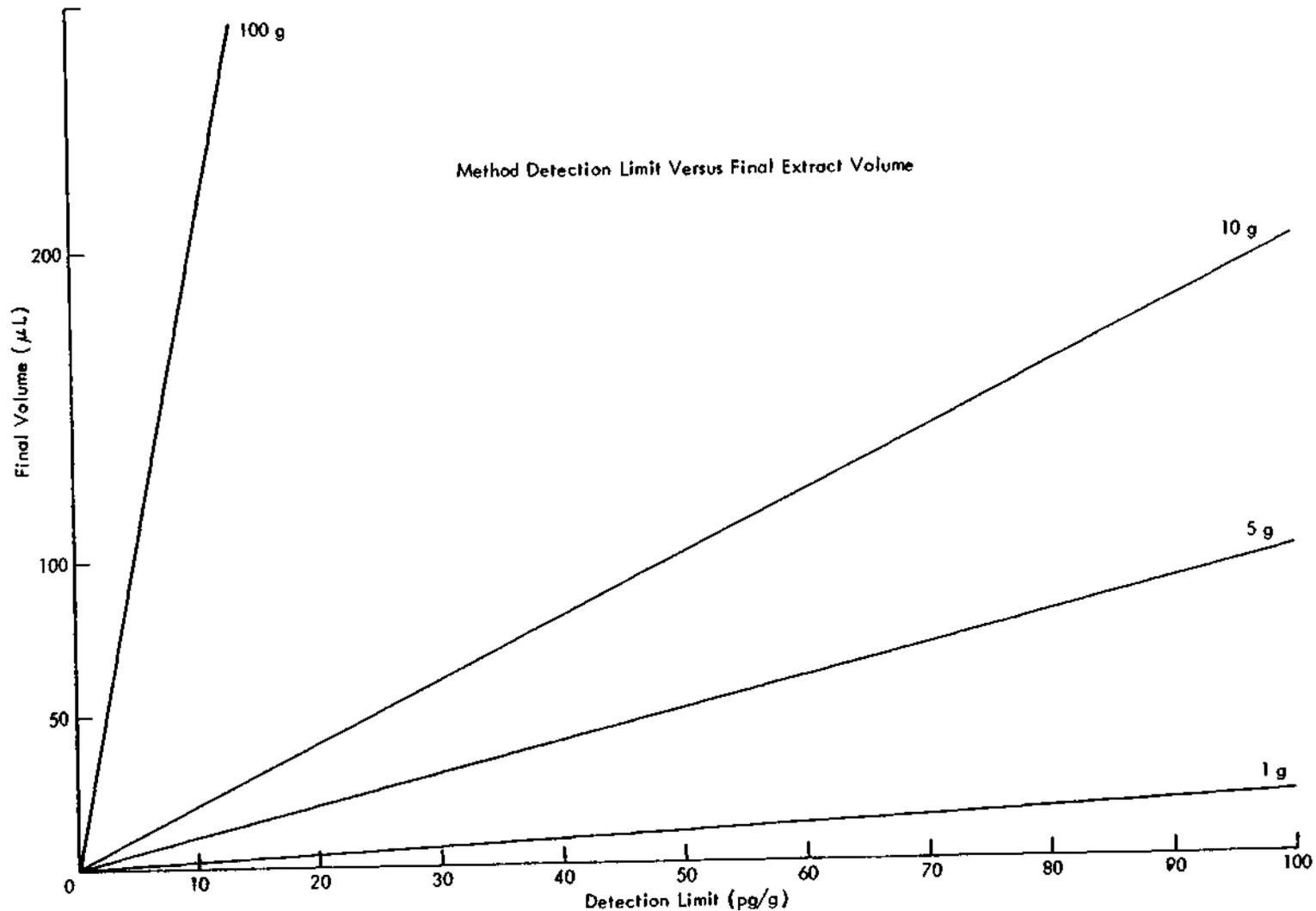
Figure 16. Method detection limit versus final extract volume and initial sample size assuming a GC/MS instrumental detection limit of 5 pg/µl on-column.
