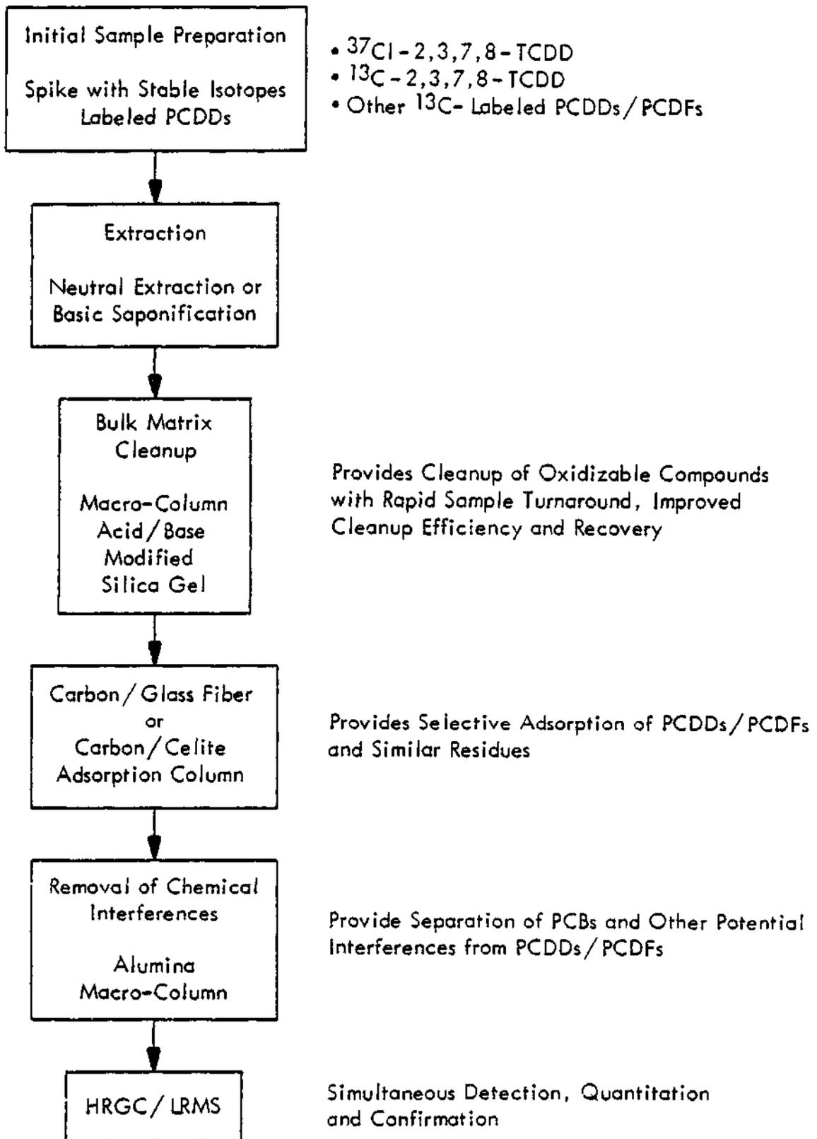
Figure 20. Schematic of proposed analytical method using low resolution mass spectrometry (LRMS).
