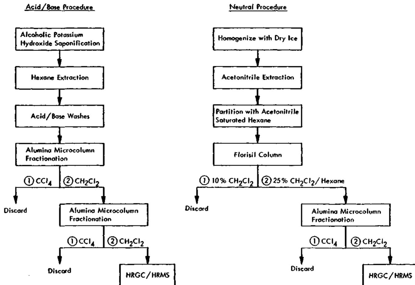
Figure 2. Schematic of EPA sample preparation procedures for preparation of biological matrices for TCDD analyses.
