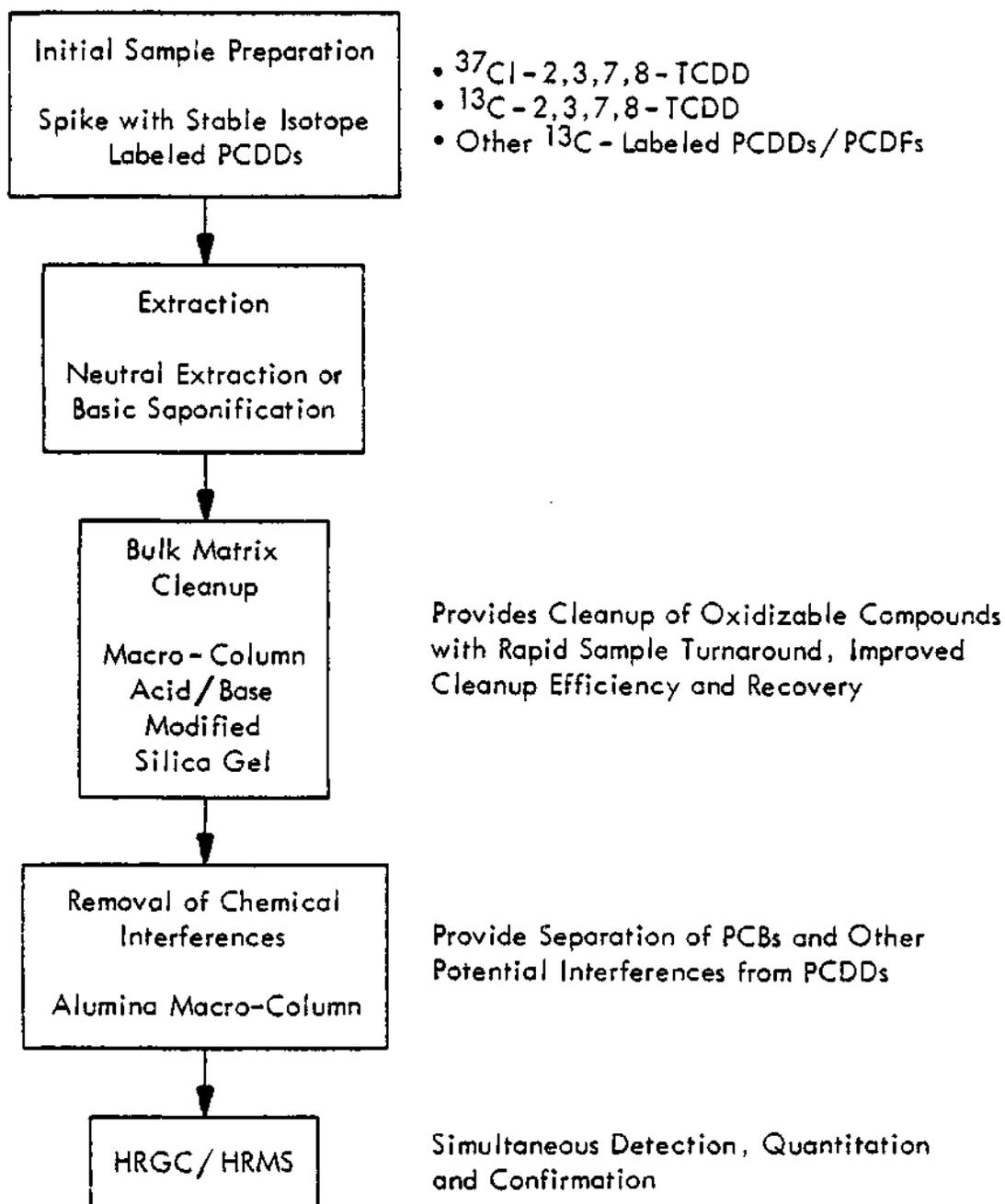
Figure 19. Schematic of proposed analytical method using high resolution mass spectrometry (HRMS).
