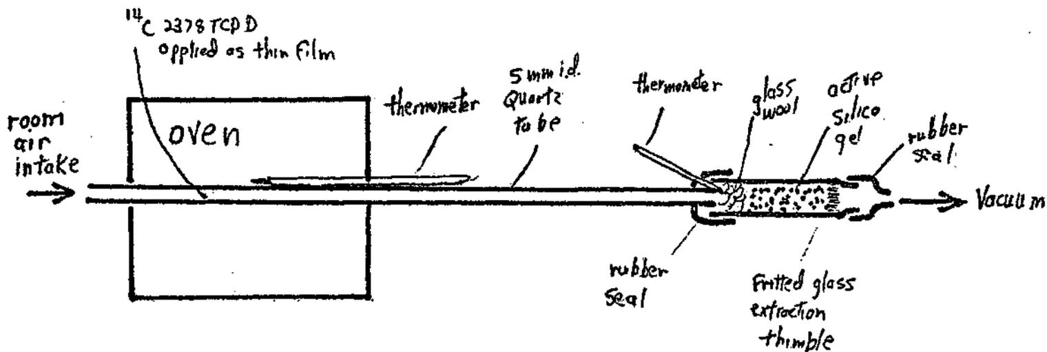
Figure 1. TCDD Volatilization and Trapping Apparatus
