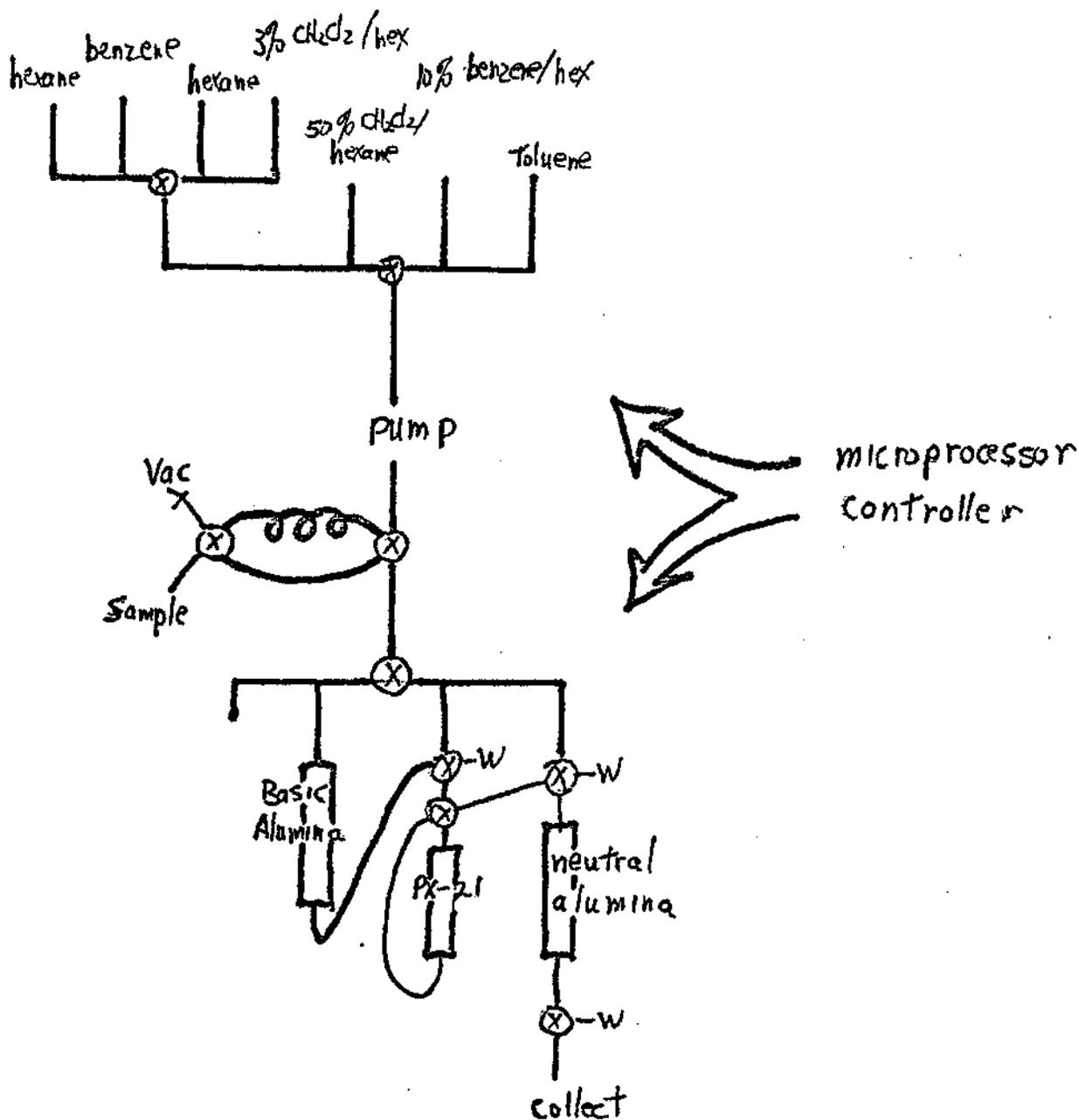
Figure 3. Automated Cleanup System For Air Samples
