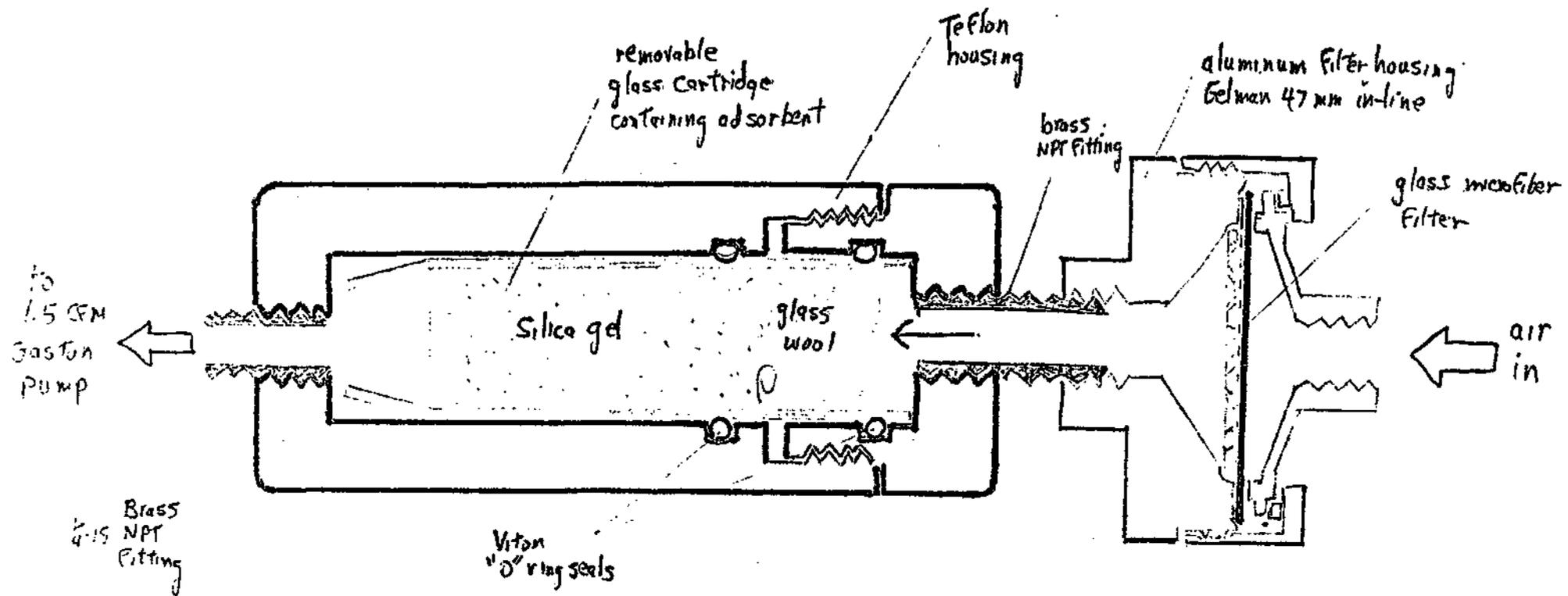
Figure 2 Two Stage Air Sampling Apparatus For PCDFs and PCDDs
