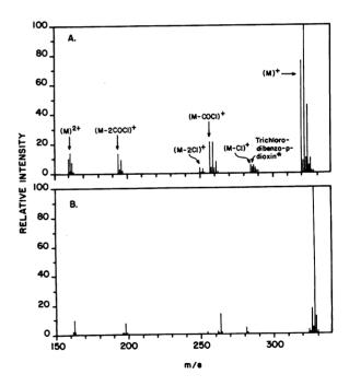
FIGURE 1. Mass spectra of (A) TCDD and (B) <sup>37</sup>Cl-labeled TCDD. The isotopic purity of the <sup>57</sup>Cl is 95.5%. The asterisk denotes an impurity. The multiplicity of lines associated with each major molecular species results from the presence of various isotopes of Cl and C.
