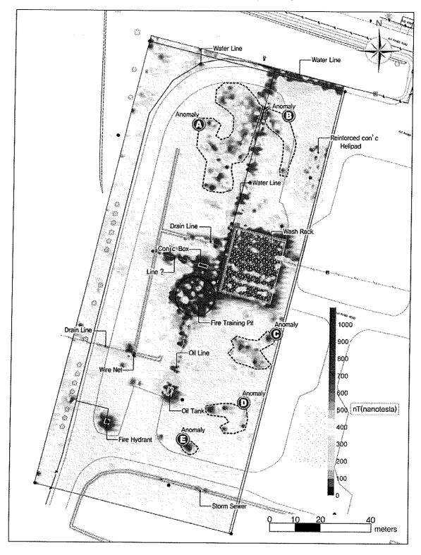
Figure 3-1. Magnetic Gradiometry Survey Result
