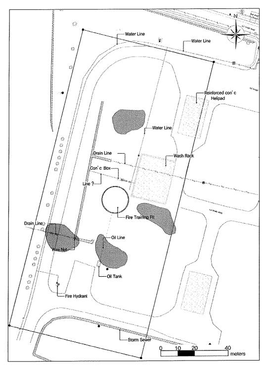
Figure 4-6 Combined Geophysical Survey Results Showing Subsurface Anomaly at Phase I of Helipad Area.
