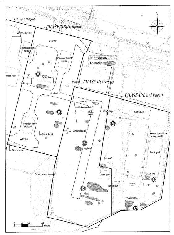
Figure 4-9 ERI Survey Result at Phase II/IIB Area.
