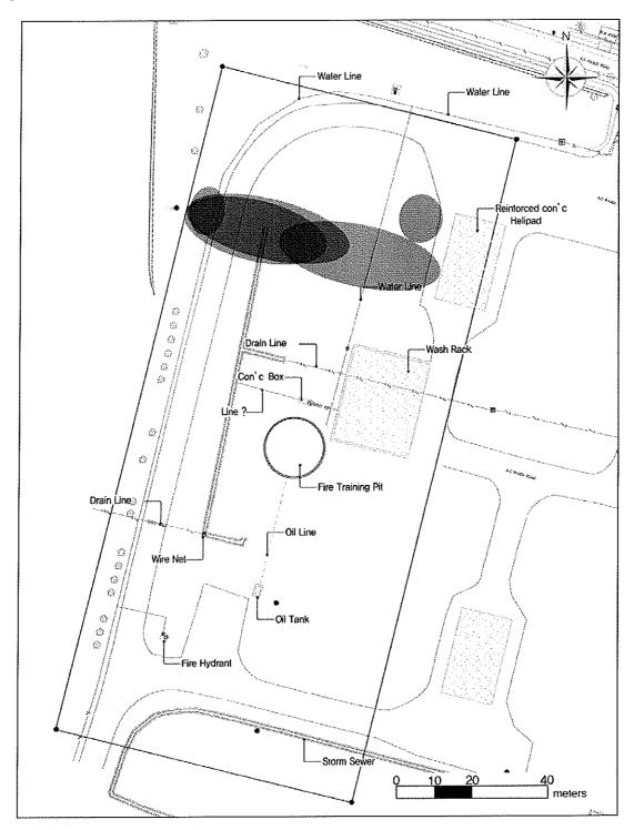
Figure 4-5 ERI Survey Result at Phase I of Helipad Area.
