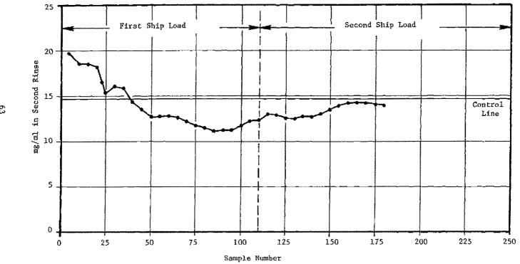
FIGURE 16. DRUM RINSE-QUALITY CONTROL CHART, RUNNING AVERAGES (47 mg/ml cutoff on high end = 179 g/gal)
